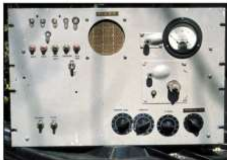
The K6MYK repeater control receiver. It was on 421.28 MHz and was built around an old military ASB-7 receiver with light-house tubes in the front end.
