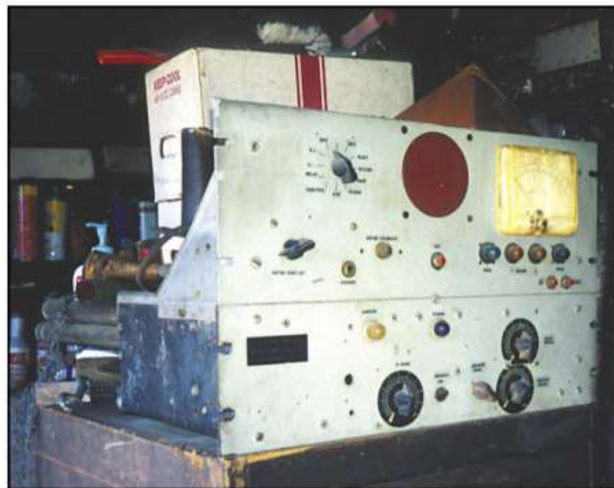
The original K6MYK AM repeater receiver.
